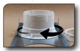
3) Optional - The riser tube is equipped with a compression ring for 4" metal conduit. If the installation requires conduit, losen the compression ring, slide the conduit into place and tighten the ring by hand until firm. CTS recommends the use of grid wire support when using conduit during the installation process.
